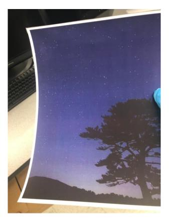
9. Place the laminated piece of paper back in the printer. Turn on only ONLY the foil layers. Turn OFF the CMYK print. Foil should be printed with black in order for the foil to stick to it best. The black stars in this print are what is going to be foiled.
