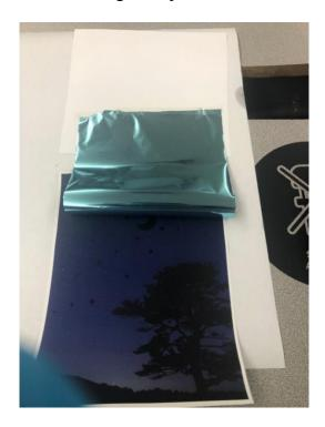
11. Set the temperature to highest setting for foil, 265 F. The speed should be set to a slow speed between 2–3.
