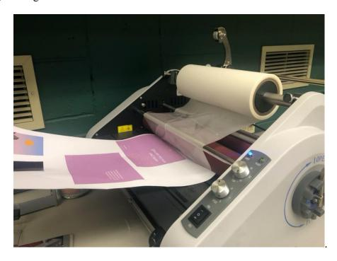
7. Set the pressure to 1 mm as pictured. Most paper will be set to 1 MM. Thicker Papers can be set to 1.5 MM.
